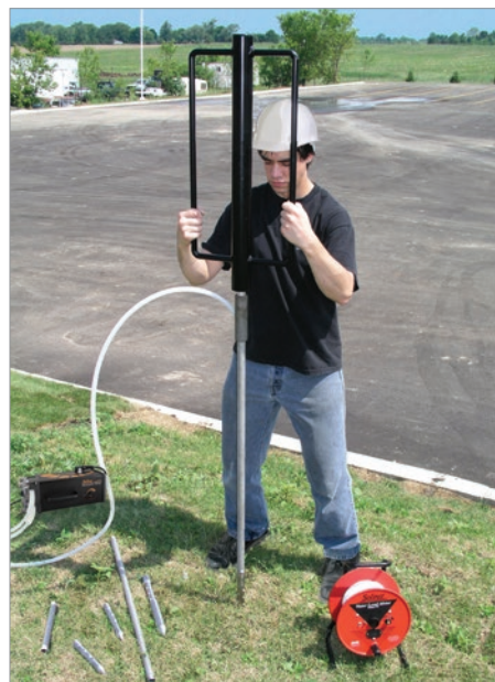
Installing Piezometers with a Manual Slide Hammer
