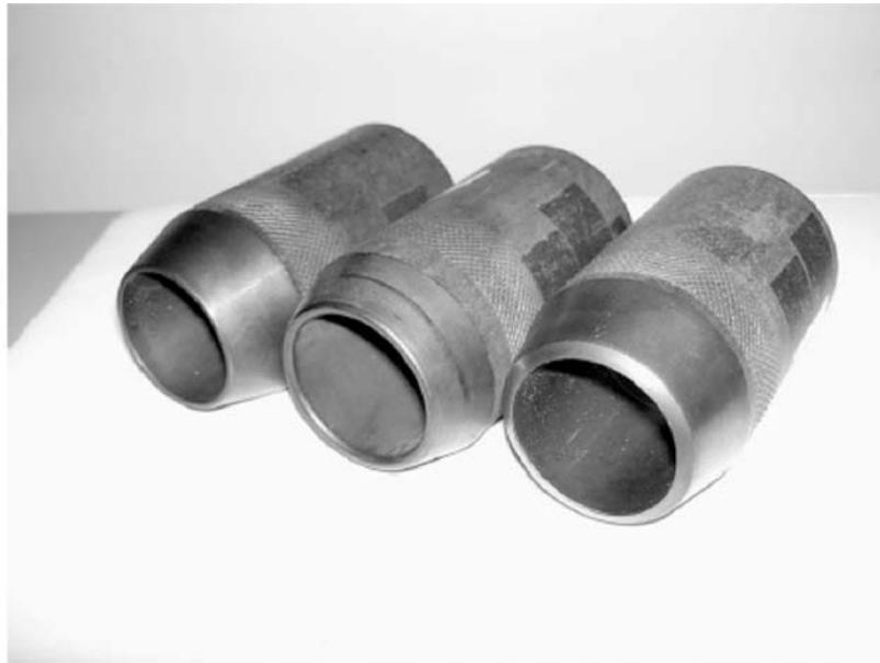
Drive samplers usually employ three types of cutting heads, or shoes, shown here. The sharp tapered heads are intended for soil sampling, while the more blunt tips are designed for greater longevity when sampling granular soils.
