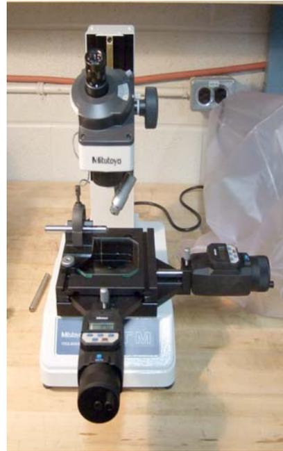
FIG. 2 Toolmaker’s Microscope
